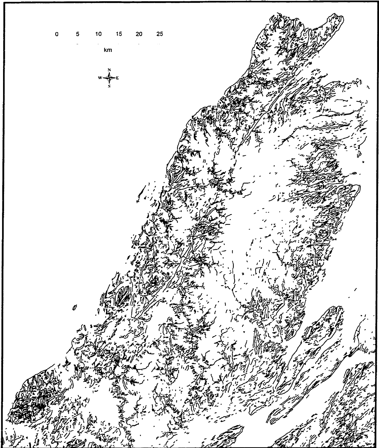
Fig 3.12 Lineaments extracted from the shaded relief digital elevation model (DEM).
