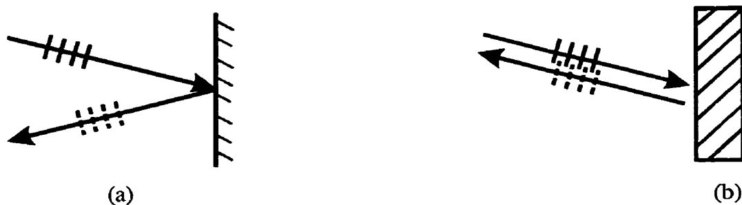
Figure 6.1 Reflection of a plane wave from (a) an ordinary mirror and (b) a phase conjugate mirror.
