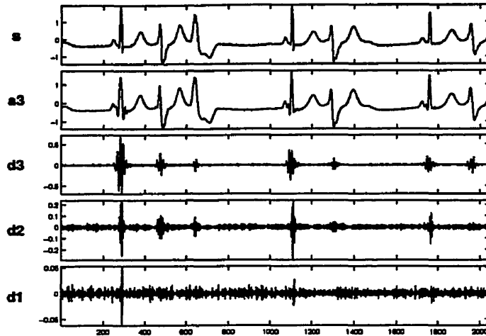
Figure 2.8: Three level wavelet decomposition of an ECG signal from record 106 of the MIT-BIH database. Here a Daubechies 10 wavelet has been applied. The scaling function associated with this wavelet has an approximation order of 10. That is, the scaling function can exactly represent a polynomial of order less than 10.
