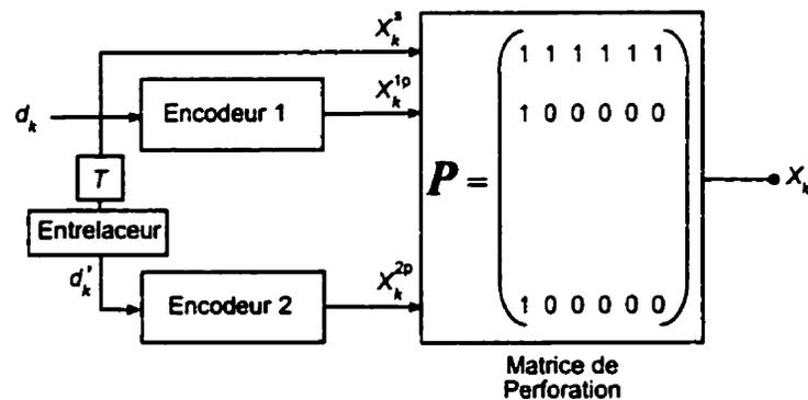
Figure 5.1: Encodeur turbo perforé à  $R_{gp} = 6/8 = 3/4$
